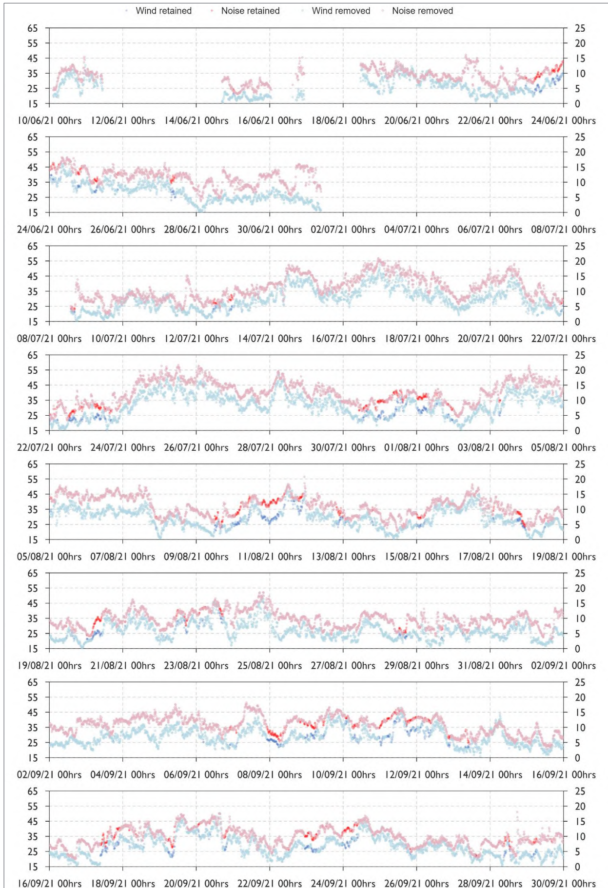
Figure 24: Intermediate J - post construction A-weighted noise level and wind speed time history
