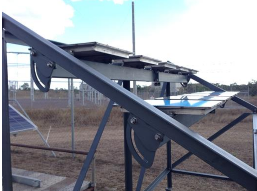
Figure 63. The test bench for dust collection on different mirrors installed at Collinsville
