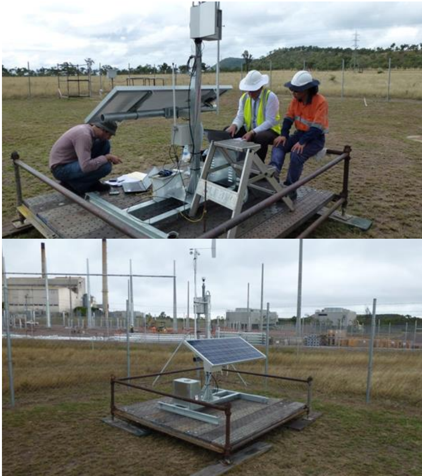
Figure 19. The dust monitor installed in Collinsville
