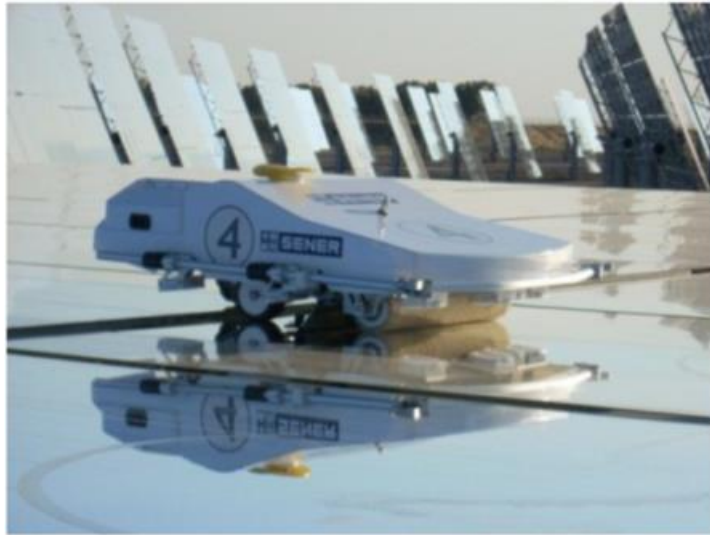
Figure 11. Cleaning robot operating in GEMASOLAR (27)
