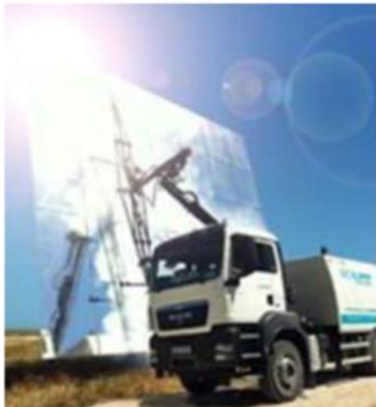
Figure 10. High-pressure water truck cleaning system (27)
