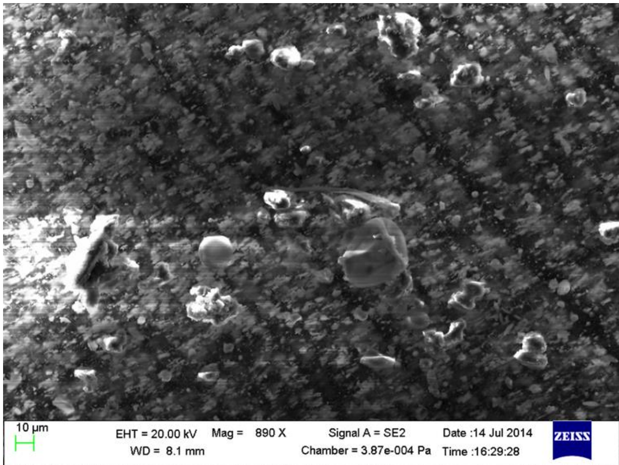
Figure 54. Electron image based on the dust sample collected in April 14
