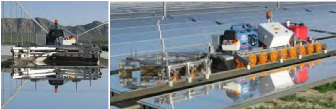
Figure 16. Novatec cleaning robot for Fresnel mirror (32)
